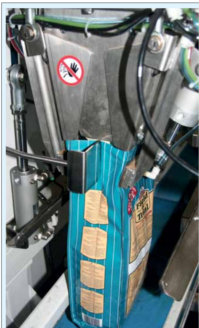
The TBC easily handles paper, plastic, woven polypropylene, hessian and nets.
